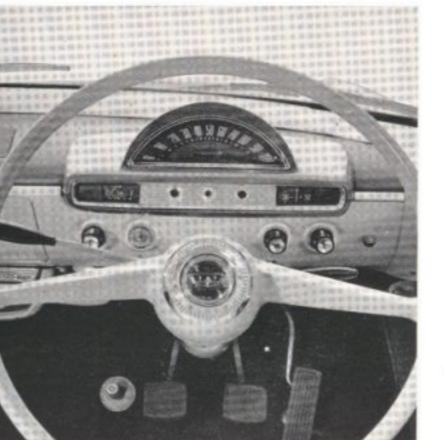
The easy-to-read instruments of the Consul are grouped in this neat binnacle directly in front of the driver.
