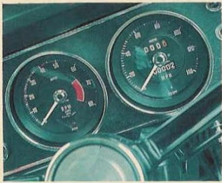
The carefully-planned facia houses a comprehensive array of instruments including a unique tachometer, calibrated speedometer and trip meter.
