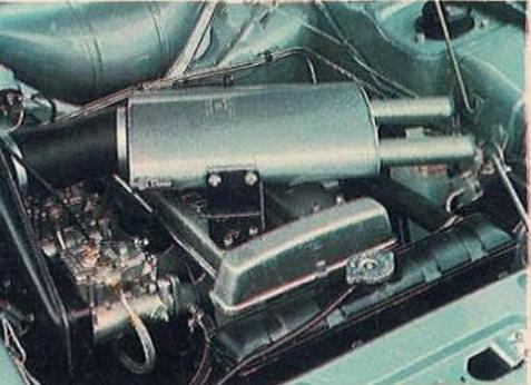
The engine is a 1558 cc version of the five bearing crankshaft Cortina engine developed by Lotus. It features light alloy cylinder head, with twin overhead camshafts, two twin-choke Weber carburettors and develops 115 bhp (gross) at 6000 rpm.
