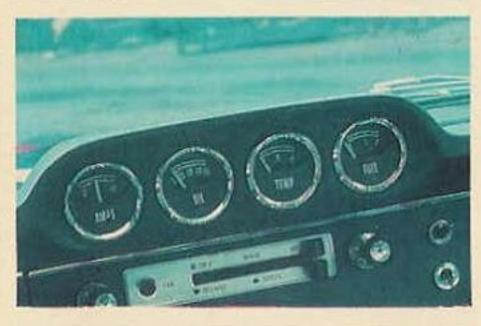
The hooded instrument binnacle has an ammeter as well as fuel, temperature and oil pressure gauges.
