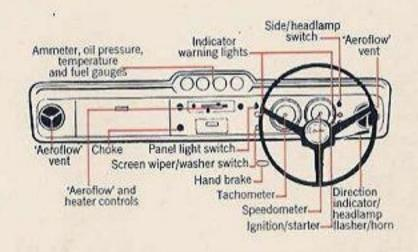
Controls: Side and headlights controlled by toggle switch on facia. Second toggle switch on the facia controls panel light. Wiper/washer, choke, ignition/ starter controls, facia mounted. Single antenna switch controlling the direction indicators, main and dipped beams, horn and headlamp flasher.
