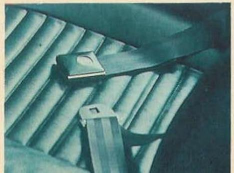
Pillar mounted seat belts are fitted as standard equipment on the Cortina Lotus. FoMoCo inertia reel seat belts are available at extra cost.
