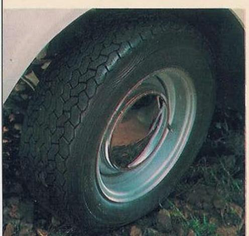
165 radial ply tyres on 5½ J rims are fitted as standard equipment. The extra wide track gives powerfully firm traction on every kind of surface at all speeds.
