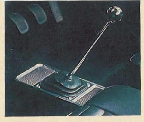
Cortina Lotus has an all-synchromesh gear box. The remote gear lever is floor-mounted for fast, easy changing.
