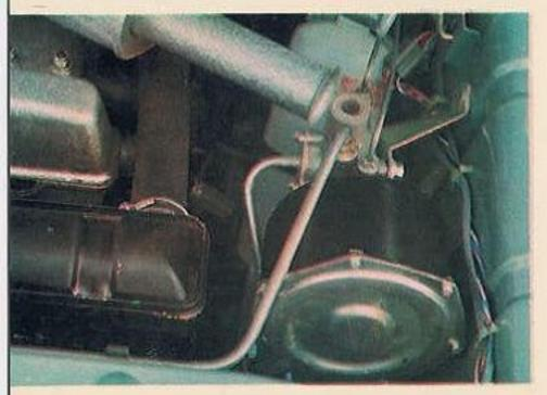
The disc brakes in front measure 9.62 inches in diameter. The self-adjusting drums at the rear are 9 inches X 1.75 inches. All brakes are servo-assisted for maximum response, maximum safety and maximum stopping power.
