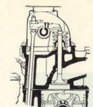
Very large OVERHEAD VALVES . . . separate inlet ports . . . ideally-shaped symmetrical combustion chamber. Result: smooth, silent running and more power from every tankful of fuel.
