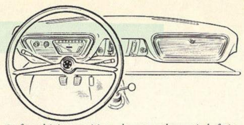
Perfect driving position—elegant and practical facia, safety steering wheel and twin padded sun visors, short sports-car type gear lever, pendant foot controls . . . . plus lockable glove box and car-wide parcel tray. Controls clearly marked with visual symbols.
