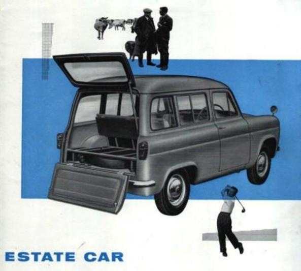
Exceptional loadspace is a big feature of the Escort—remarkable for so compact a vehicle. And it's very accessible too, thanks to the wide-opening lightweight tail-gates. Fold forward the rear seat for maximum loadspace. The floor space is stressed for loads up to 5 cwt., and the rubbing strips on the floor allow heavy loads to be slid in and out with the greatest of ease.
