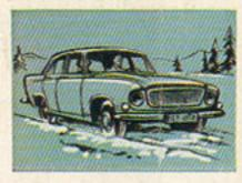
4 cylinder in line O.H.V. Capacity 1703 c.c. (103.9 cu. ins.), Bore 82.55 mm. (3.25 ins.). Stroke 79.5 mm. (3.13 ins.). Maximum Gross B.H.P.
