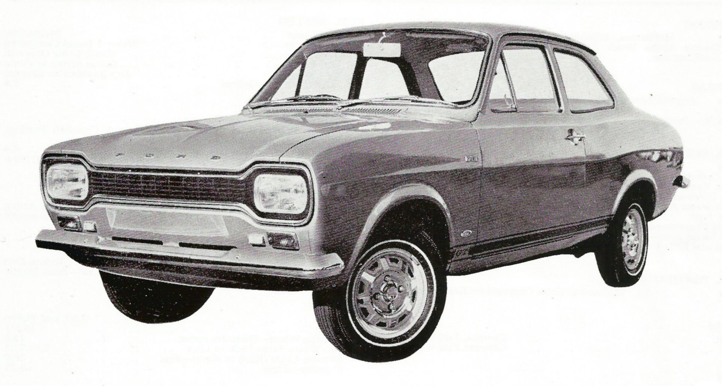
The sporty appearance of the Escort G.T. is endorsed by the car's peppy performance. Its engine is fitted with a Weber 2 barrel carburettor and develops 75 Brake Horse Power. Full instrumentation is standard.
