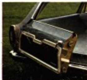
Magic Doorgate opens as a door and as a tailgate.
