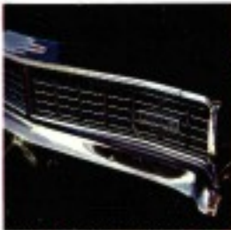
Retractable headlamp doors open as lights come on.
