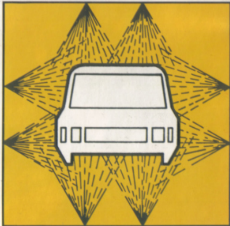
Spray System to cover both inside and outside of vehicle.
