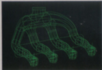
To make full use of the helical swirl characteristics of the intake ports an extremely sophisticated inlet manifold was developed in a computer-aided design study.
