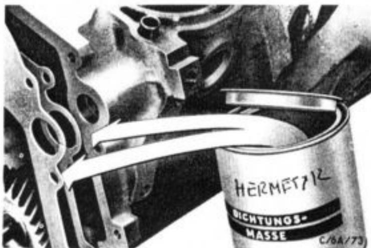
Note ! The outer rim of the two large holes in the front intermediate plate has been provided with a slit to ensure that in case of a defective seal ring the coolant flows out of the engine and not into the oil pan. It is essential that defective seal rings be replaced immediately.
