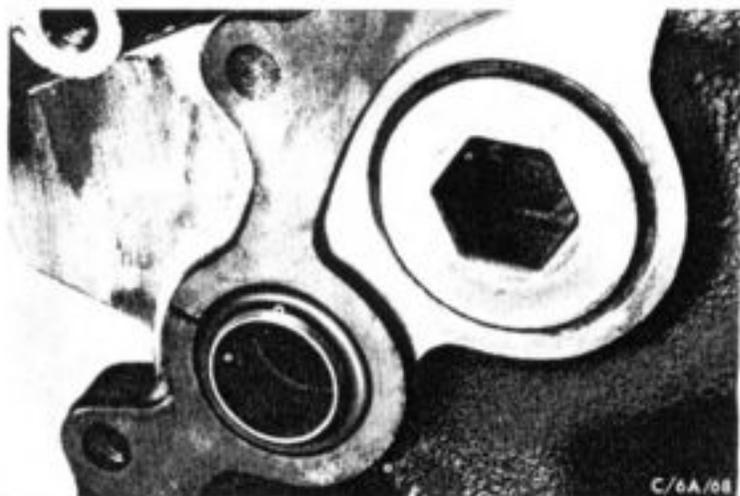
Apply sealing compound to both sides of the front cover gasket and stick the gasket onto the intermediate plate. Position the front cover and initially fingertighten it with two screws. Slide V-belt pulley with fitted tool GC 6059-A onto the crankshaft. Fit and slightly tighten the retaining bolt and washer to centralize the front cover to the crankshaft. In this position fit and torque the front cover retaining screws to specification. Then remove the pulley and take off the tool.
