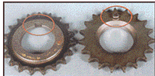
The original crank gear (right) had a small, raised tab sticking out from the back side of the gear that fit into the notch that was machined in the crank. The later design had a slot machined in the gear for a Woodruff key.
