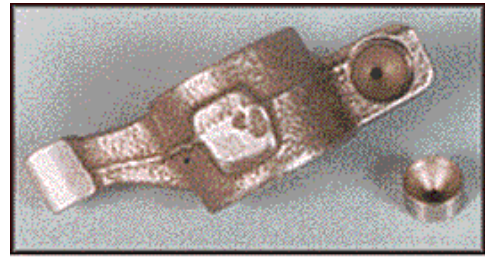
The worn pushrod socket in the rocker can be repaired by installing a new insert in the rocker. The rocker in the picture has been rebuilt with a new socket.
