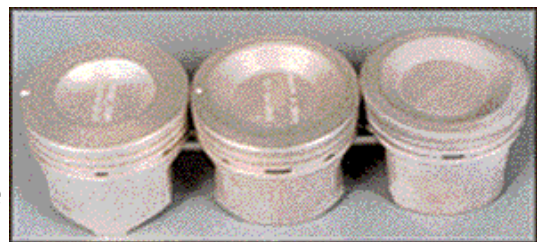
There have been three pistons used in the 4.0L. The original design (left) had a shallow dish, the second version (middle) had a deeper dish to compensate for them smaller, heart-shaped chamber, and the latest design (right) had a similar dish, but it was more squared-off in the bottom.
